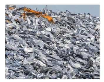
As a highly recyclable metal that is used in many industrial sectors, aluminum is a crucial link in the circular economy supply chain. To achieve the right mix of strength, corrosion resistance, and other desirable properties, manufacturers create aluminum alloys with differing elements. However, with each round in the repeated melting and reuse of aluminum alloys, impurities such as iron, copper, zinc, magnesium, silicon, and manganese accumulate.
