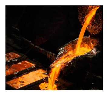
A key sustainability benefit of aluminum is its ability to be melted and recast repeatedly, making it inherently recyclable. Recycling aluminum is an important way to avoid greenhouse gas emissions, since processing secondary aluminum takes only a fraction of the energy needed to make new metal from its ores.<sup>1</sup>
