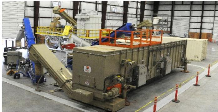
*The Process Development Unit (PDU) is a modular, fully integrated, full-size biomass preprocessing system for design and scale-up of bioenergy facilities. The PDU offers toll processing, piloting, third party equipment testing and preprocessing R&D. The PDU has a maximum process rate of five tons per hour and allows partners to test grinding, drying, pelletizing, cubing, torrefaction, and mechanical and chemical separation options.*
