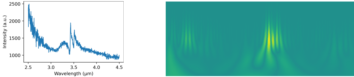
(a) Raw MIR spectrum of PE measured at 30 ms (2.5-4.5 \mu\text{m} ). (b) CCWT scalogram of PE spectrum used as 2D CNN input.
