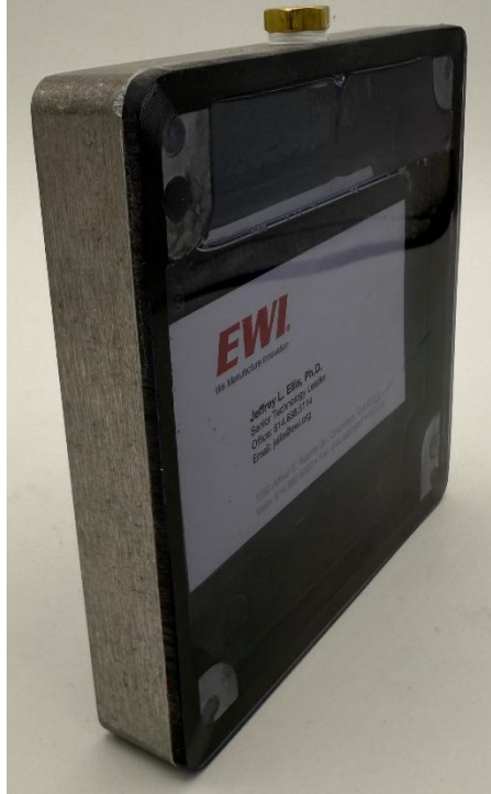
Figure 8. PVC-to-aluminum joint container holding liquid to demonstrate a hermetic seal
