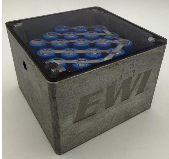
Figure 4. PVC top-to-aluminum battery enclosure
