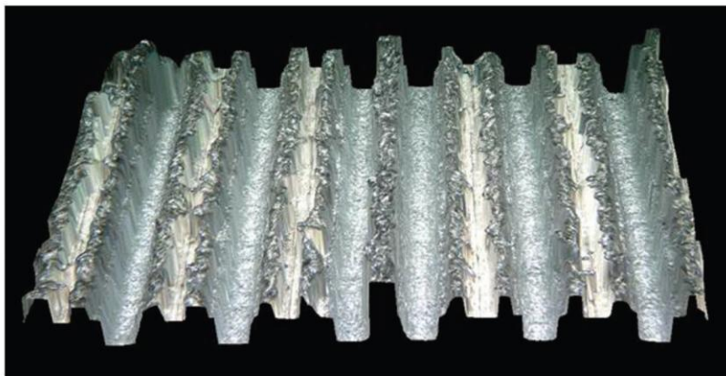
Figure 1. Confocal scan of valleys (~60 \mu\text{m} feature depth) with overhanging fingers or bridges on etched aluminum
