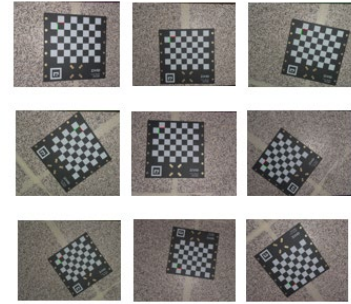
(c) Checkerboard images for calibration
