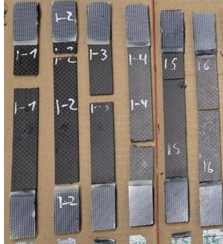
Figure 5: Tensile test specimen with tabs after testing
