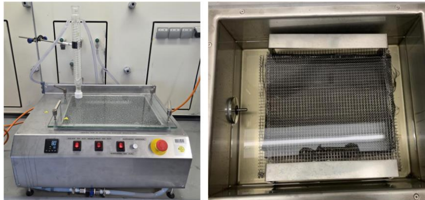
Figure 3: Recycling unit (left), permeable clamping elements (right)
