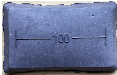
Figure 1. Example of compression molded foam with 100 mm imprint.
