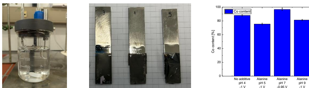
Figure 7: Image of the used cell for Co deposition. Center: Deposits of Co/Ni. Right: Cobalt content of the deposit dependent on varying parameters with added alanine.
