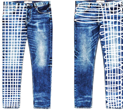
Figure 5: On the left, current jeans made of many short lengths of horizontal weft yarn, as the fabric is stamped when cutting pattern pieces; on the right, our technology allows for jeans to be made from a continuous single weft yarn, skipping the stamping stage
