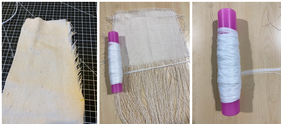
Figure 6: Process of removing weft yarn from a Vega 3D woven pant, keeping the yarn intact
