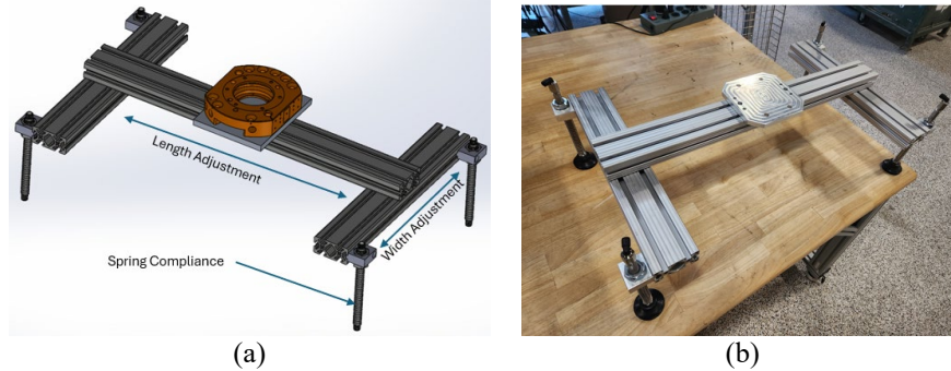
Figure 8: Suction gripper system (a) CAD design (b) built gripper.
